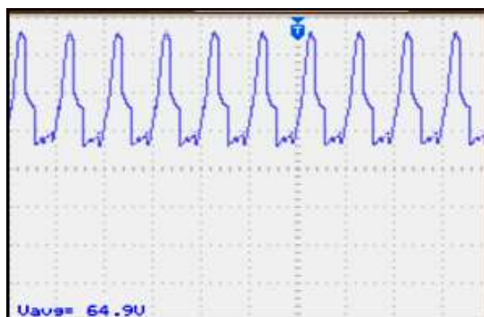
Fig -7: Output voltage V_d for 12-pulse converter when \alpha = 60^\circ for R Load without filter
