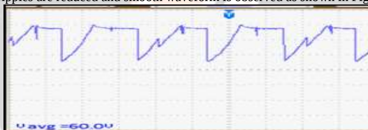
Fig -9: Output voltage V_d for 12-pulse converter when \alpha = 60^\circ for RL Load without filter
