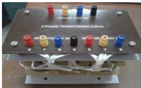
Fig -4: Three phase 500VA converter Transformer
