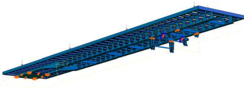
Figure 3: Static load (pressure=67564.5N/m 2 )
