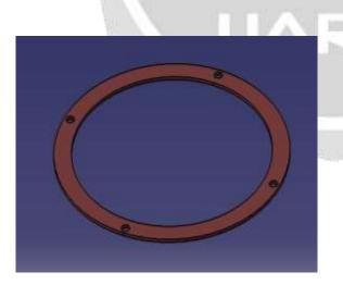
Minimum Contact Pressure, Pc=Pi×[(G/4b)+m]
