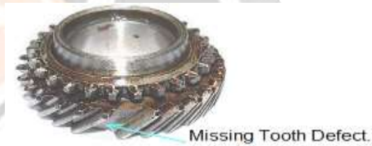
Fig-6. Sample of Defective Gear: Missing Tooth defect
