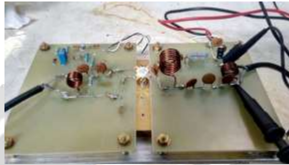
Figure 9: View of the 25W SSPA hardware
