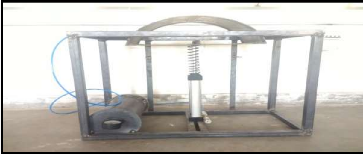
Fig-9. Set Up of Speed Breaker Device For generation of Compressed Air by Using Spring Suspension System
