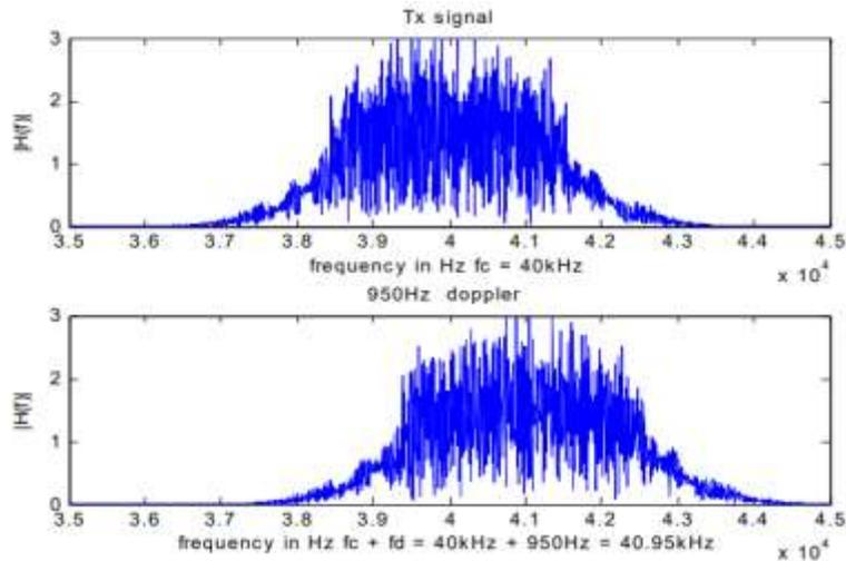
Fig -5 Spectrum displacement due to 950Hz at 40kHz
