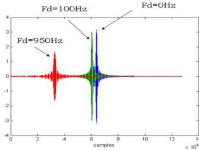
**Fig -8 Matched Filter output with up chirp**
