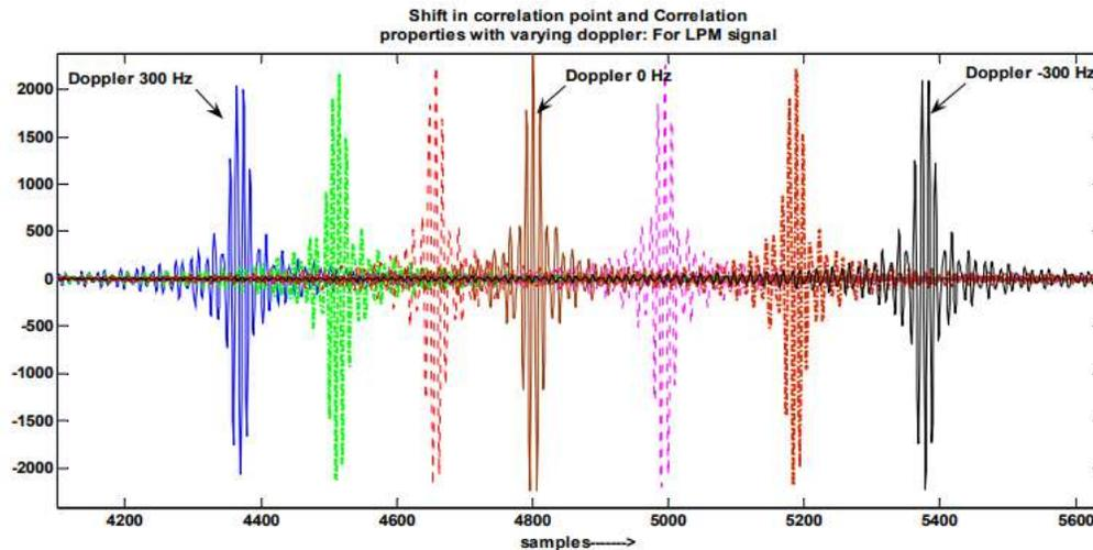
**Fig-1: Correlation characteristic of LPM signal with its Doppler shifted version**
