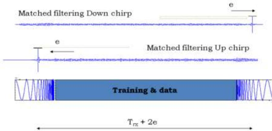
**Fig -10 Increase in Trx due to shifting of chirp**
