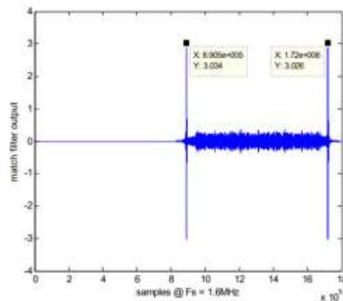
**Fig -7 Matched Filter output with up chirp**
