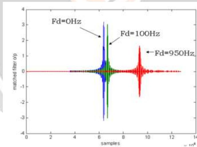
**Fig -9 Matched Filter output with up chirp**
