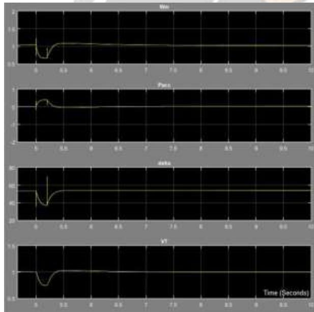
Figure 14. When applied at the end of the transmission line for BGPP, one phase fault occurs at  $t=5s$ .
