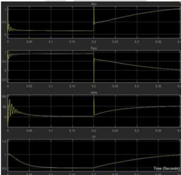
Figure 16. In Fig. 15, zoom in on the duration of a three-phase fault when applied at the end of a transmission line for BGPP.
