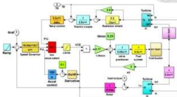
Figure 6. Controller model for a simulated gas turbine [14]
