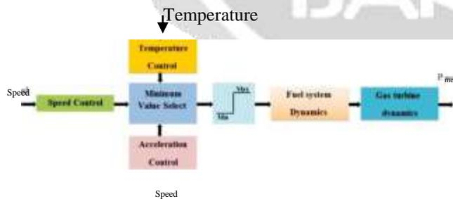
Figure 3. Reduced complexity of Rowen's HDGT model[10].
