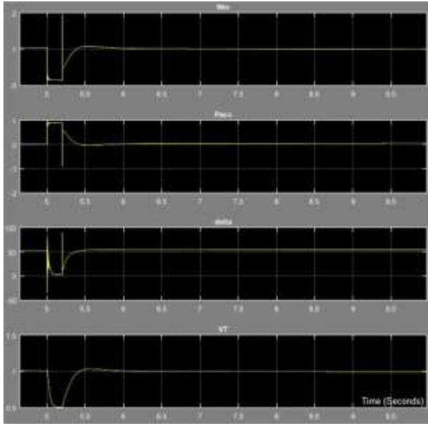
Figure 15. When  $t=5s$ , a 3-ph fault occurs at the end of the transmission line for BGPP..
