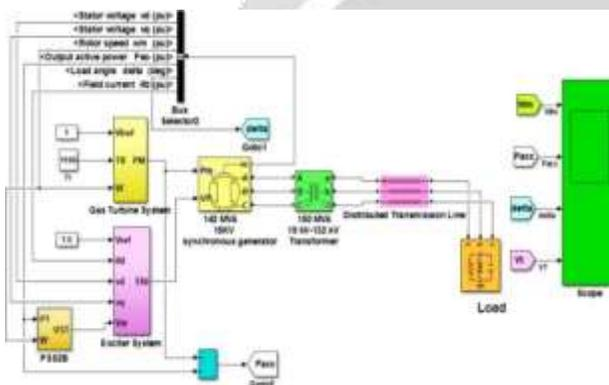
Figure 12. The model for a single unit (unit in Fig. 11) of BGPP
