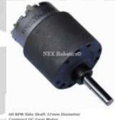
60 RPM Side Shaft 37mm Diameter Compact DC Gear Motor is suitable for small robots / automation systems. It has sturdy construction with gear box built to handle stall torque produced by the motor. Drive shaft is supported from both sides with metal bushes. Motor runs smoothly from 4V to 12V and gives 60 RPM at 12V. Motor has 6mm diameter, 22mm length drive shaft with D shape for excellent coupling.
