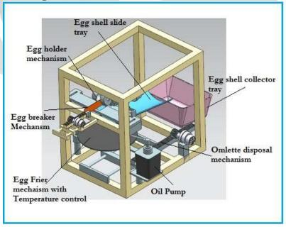
The machine has four basic system
