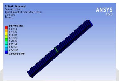
The maximum stress induced in the part material is 0.57461 MPa which is far below the allowable stress of 100 Mpa hence the rack is safe,
