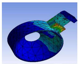
The maximum stress induced in the part material is 0.57461 MPa which is far below the allowable stress of 100 Mpa hence the rack is safe
