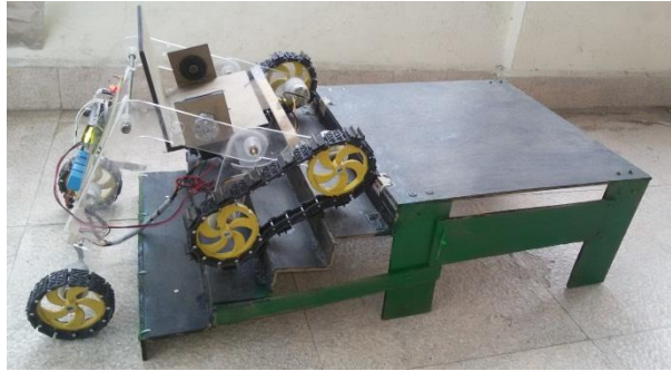
Fig-11(e): Robot climbing 4 th step in Forward direction
