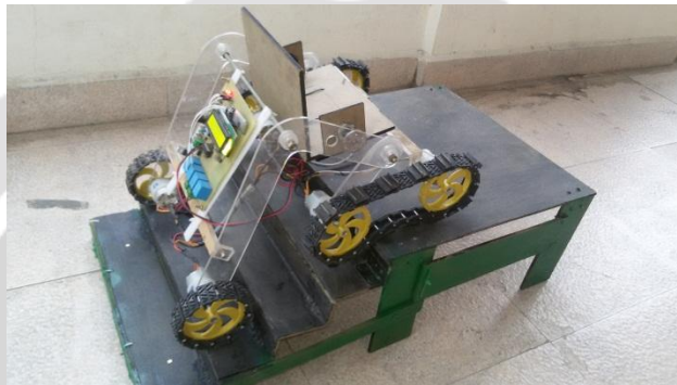
Fig-11(f): Robot climbing final flat step in Forward direction
