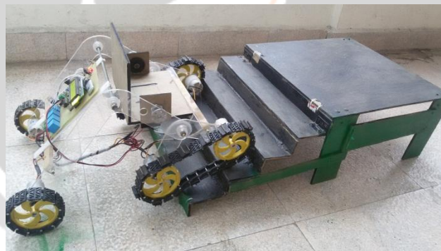
Fig-11(c): Robot climbing 2 nd step in Forward direction
