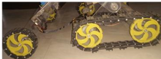
Fig-5: Wheels and conveyer belt assembly of robot
