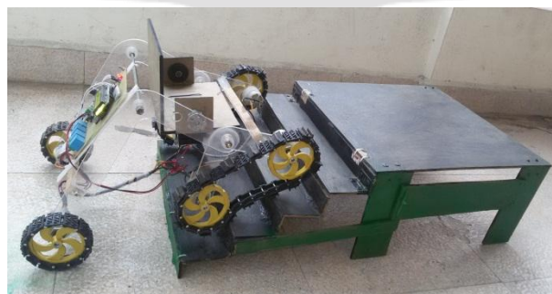
Fig-11(d): Robot climbing 3 rd step in Forward direction
