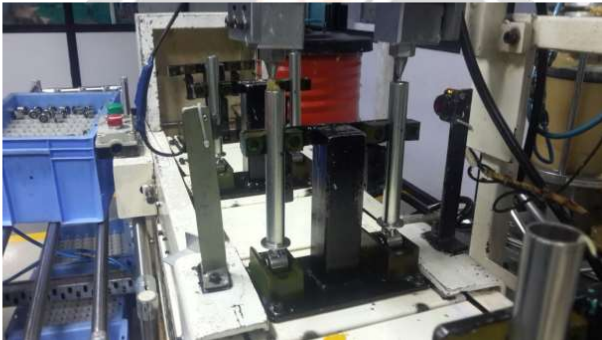
Fig 2.1. Actual Grease filling machine (Project area).
