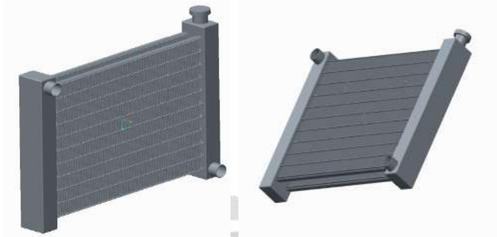
Fig.2.1.1 3D Model of Radiator using CREO
