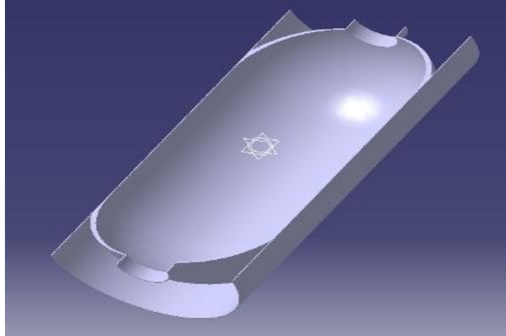
Fig -3: Sectional view of 3D model of rocket motor case
