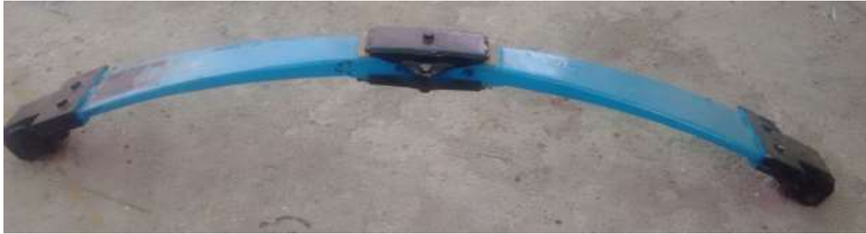
Fig. 2.1 composite Leaf spring Design
