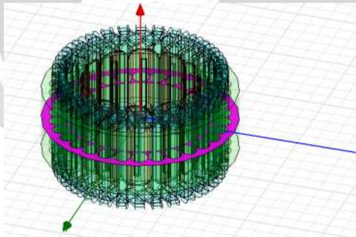
**Fig.9:** Sectioning of Stator and Rotor for Magnetostatic Analysis
