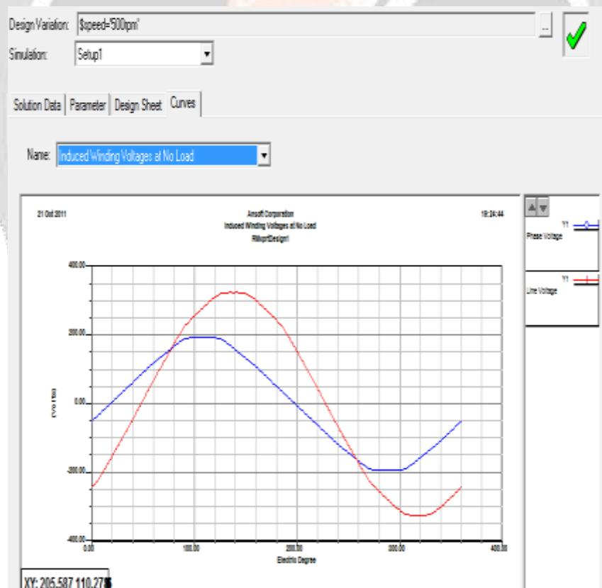
**Fig.10:** Induced winding voltage at line and phase
