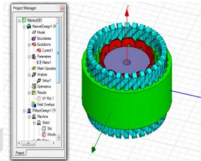
**Fig.8:** Ansoft RMxprt Construction of PMSG Export to Ansoft- Maxwell 3D Design
