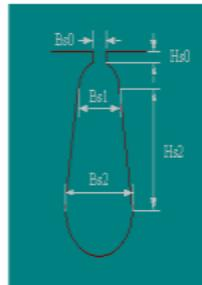
**Fig.4:**Stator slot design
