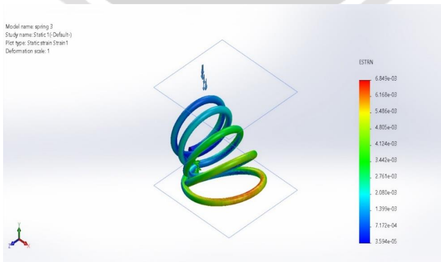
Fig. 9 The Strain in Spring Made of Steel Structure
