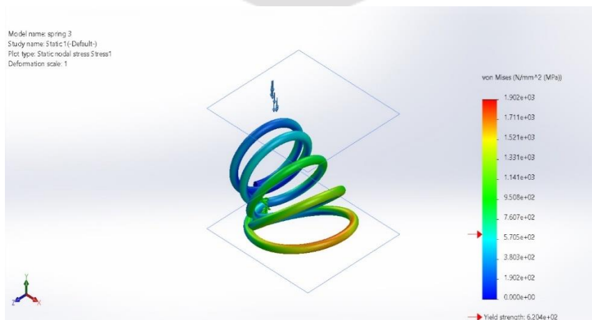
Fig. 6 The Stress in Spring Made of Steel Structure
