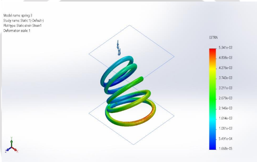
Fig. 8 The Strain in Spring Made of Copper Alloy
