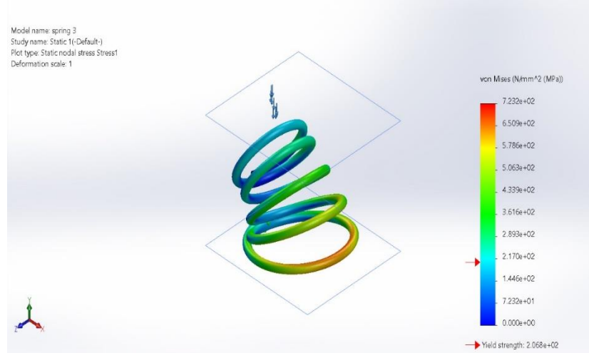
Fig. 7 The Stress in Spring Made of Copper Alloy
