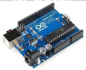
Fig-3 Arduino Uno Microcontroller
