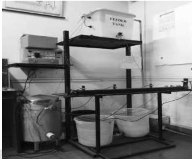
Fig -3: Experimental Setup of Bottle Filling Plant and Tank Level Control System
