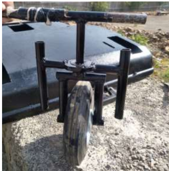
Fig-38: Steering Handle construction
