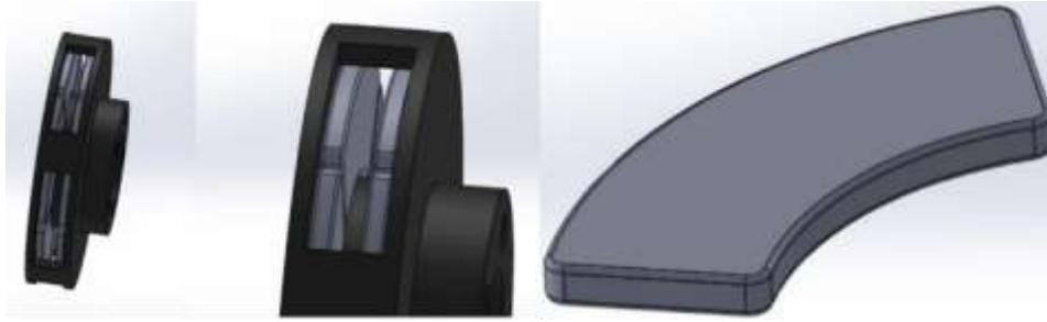
Fig -3: Installation of TEGs on the inner sides of the disc (Model by Prakhar Tonk et al [10])
