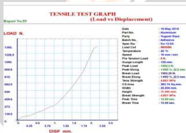
Fig.3 Load vs. Displacement graph of adhesive joint having 12.5 mm Lap length.
