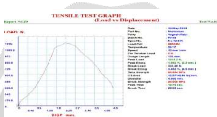
Fig. 7 Load vs. Displacement graph of Rivet joint having 12.5 mm Lap length
