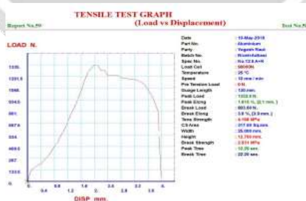
Fig. 11 Load vs. Displacement graph of Adhesive+ Rivet joint having 12.5 mm Lap length.
