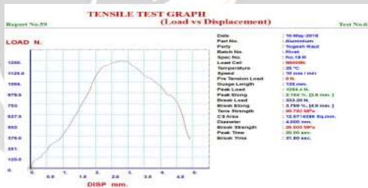
Fig. 8 Load vs. Displacement graph of Rivet joint having 18 mm Lap length.
