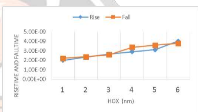
Fig.14 Variation of power with respect to oxide thickness. Fig.15 Variation of rise and fall time with respect to oxide thickness.
