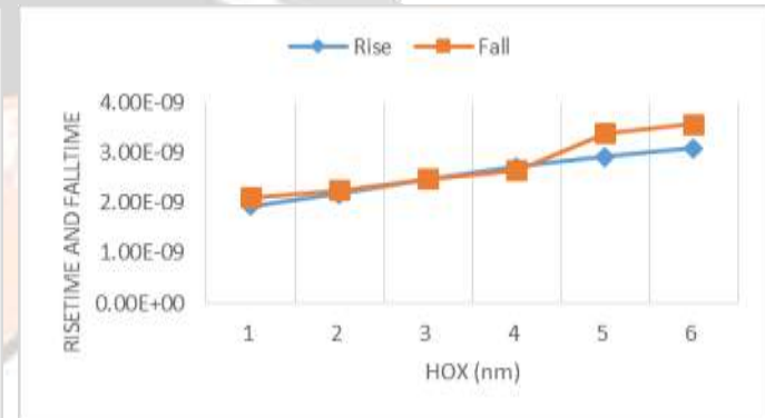
Fig. 9 Variation of rise and fall time with respect to oxide thickness.
