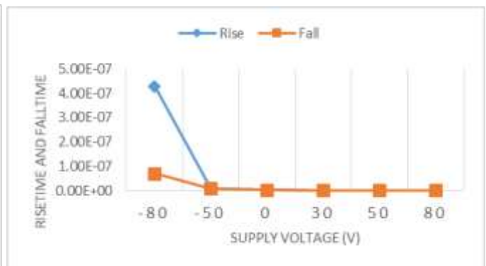
Fig. 7 Variation of rise time and fall with respect to supply voltage.
