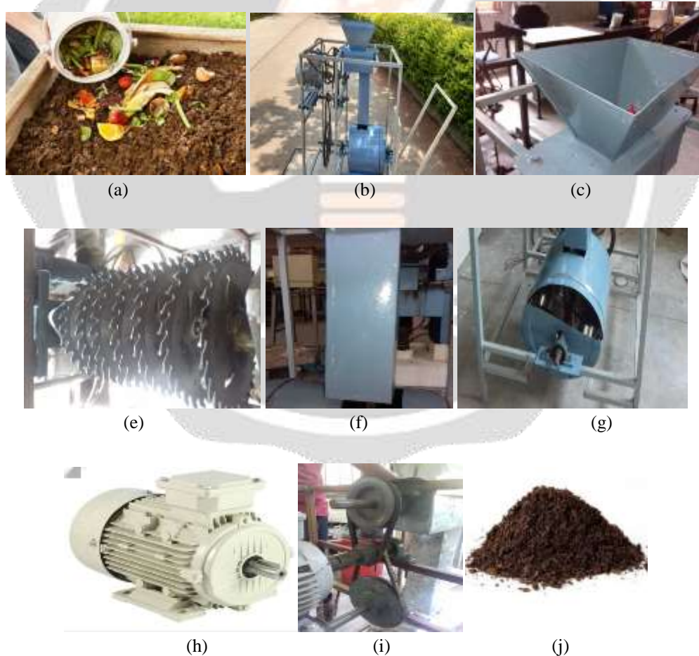
Fig. 1 Experimental setup (a) Organic Waste. (b) Model (c) Hopper (d) Saw Cutter (e) Rectangle box (f) Shredder tank (g) 3-phase induction motor (h) Pulley Drive (i) Compost
