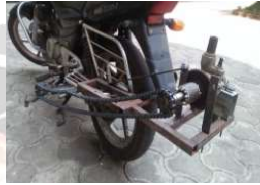
Fig 4.7 – water pump attached to motorcycle
