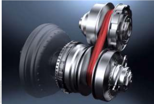
Fig-1.1: - CV TECH CVT with Primary, Secondary & Belt
