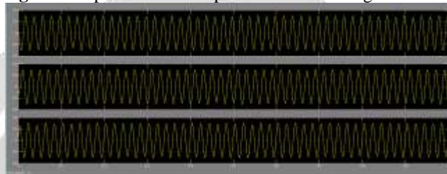
Fig 7: Three phase 3level output current waveform
