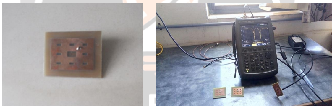
Fig. 9 Fabricated Fractal antenna with 2 nd Iteration
