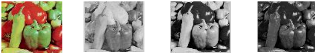
Fig 4: (a) Original Image,(b) Red Component of Original Image,(c) Green Component of Original Image,(d) Blue Component of Original Image
