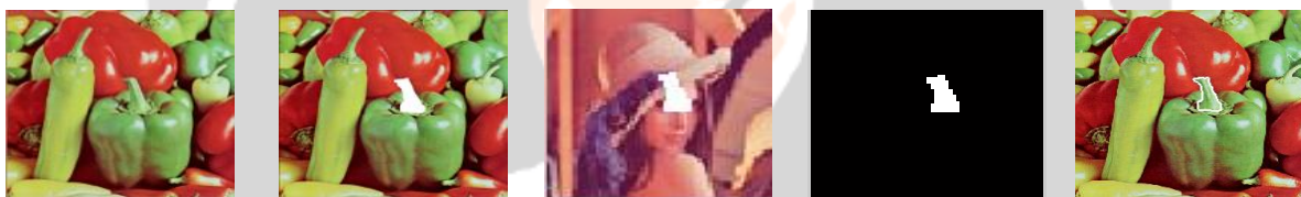
Fig 7:Deletion Attack: (a) Watermarked final image, (b)Tampered watermarked Image, (c)Tampered extracted decrypted watermark using right keys, (d) Tampered area detection after XOR operation, (e)Tampered area located in original image
