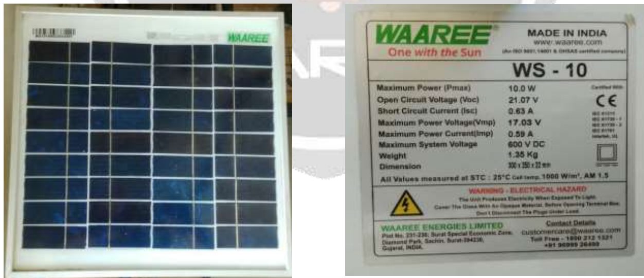
Fig- 1: Solar panel & its specification
