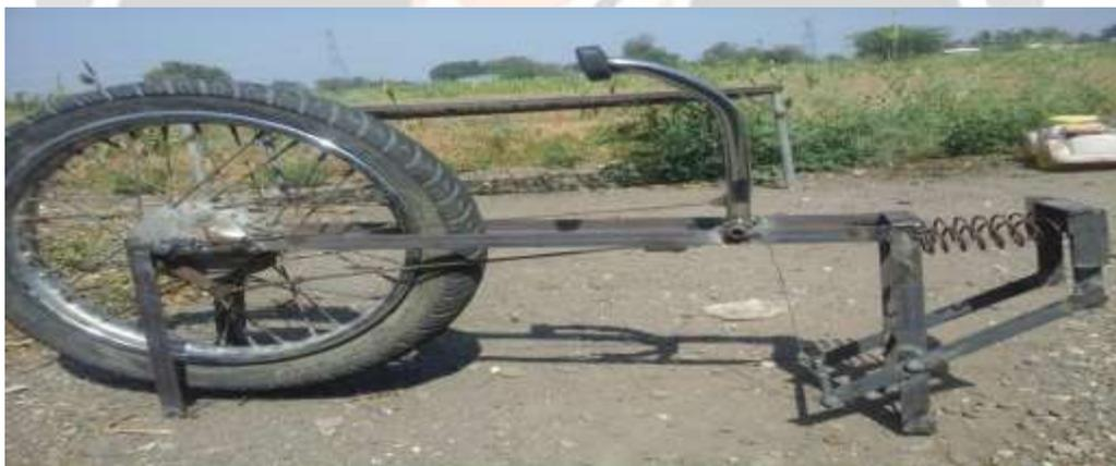
Figure shows actual diagram of project here flexible bumper is attached to the chassis of the vehicle by means of spring. Hence bumper gets compressed against spring force on the application of External force. Hence, we called this Bumper as Flexible bumper because it gets pressed under the application of external force. Hence this bumper is pressed due to any obstacle coming front of the vehicle.
