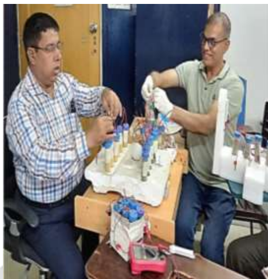
Fig.1 Experimental set-up for Ginger based LED lamp
