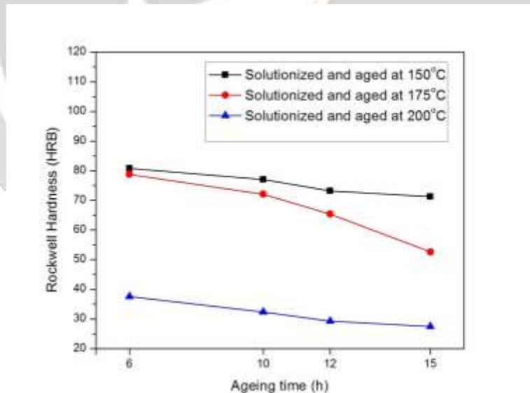
**Fig-8:** Effect of ageing time and temperature on Hardness of the 7075 Al-SiC MMC'S Solutionized at 495°C for 6h and aged.
