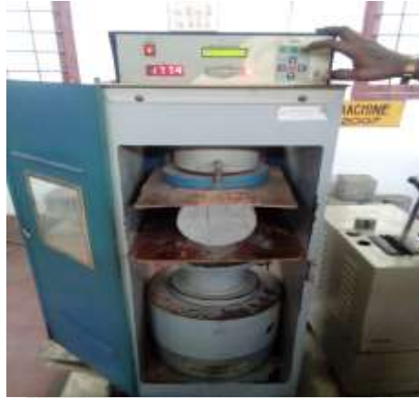
Fig- 2: Split tensile strength testing of cylinder
