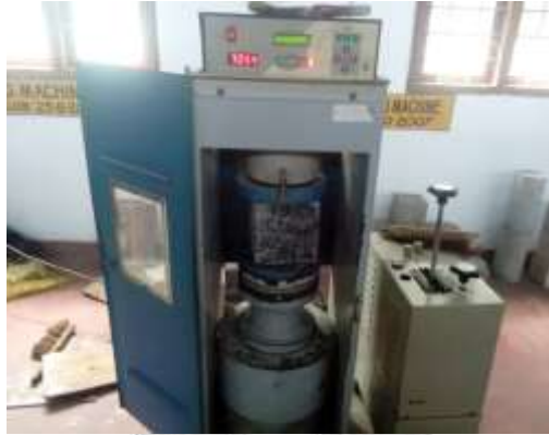
Fig- 1: Compressive strength testing of cube
