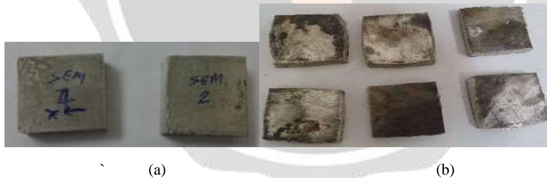
Figure 3.1: Sample (a) before forging, (b) After forging
