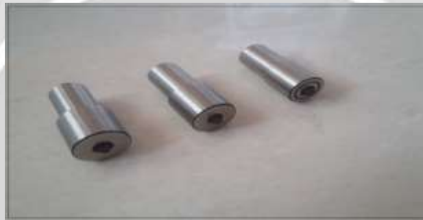
Fig -2: Three tools with shoulder to pin diameter ( D/d= 5.5, 5.0, 4.5 ) ratio
