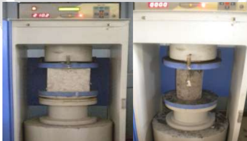
Fig.3 Compressive Strength Test
