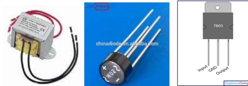
Fig -11 Transformer, Bridge rectifier, Regulator IC
