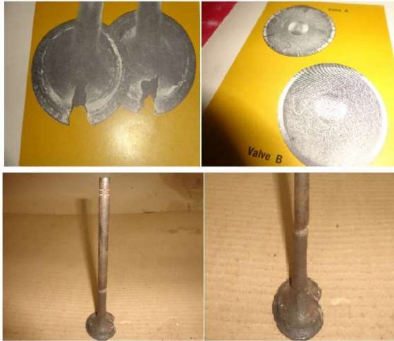
Fig.3failure due to high temperature
