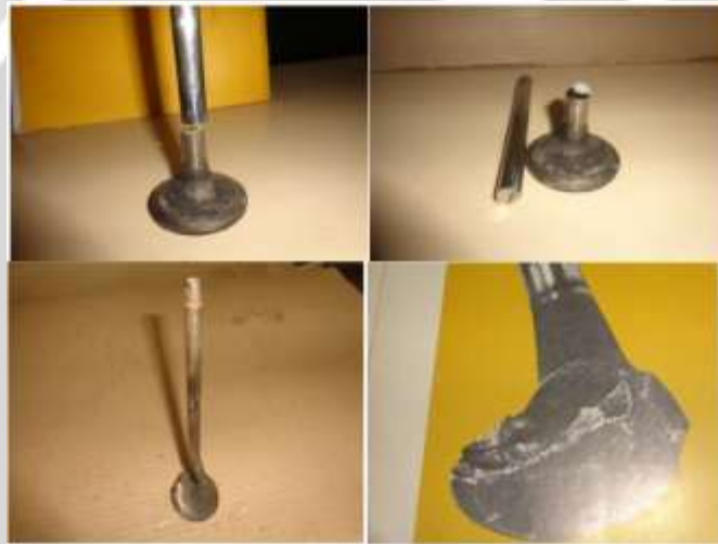
Fig.2 Valve failure due to fatigue
