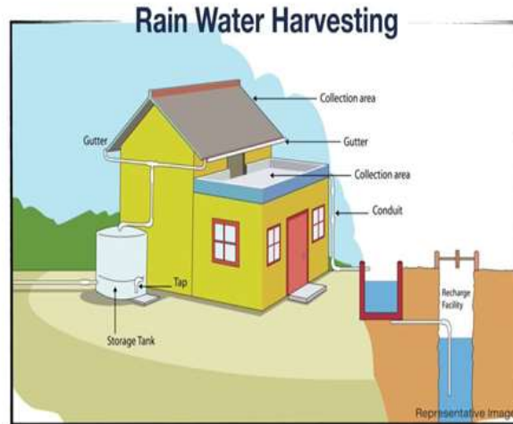
Fig -1: Components of Rainwater Harvesting
