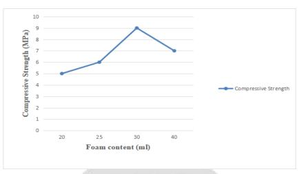
and then decreases the strength of block so optimum content is chosen which is shown in graph
