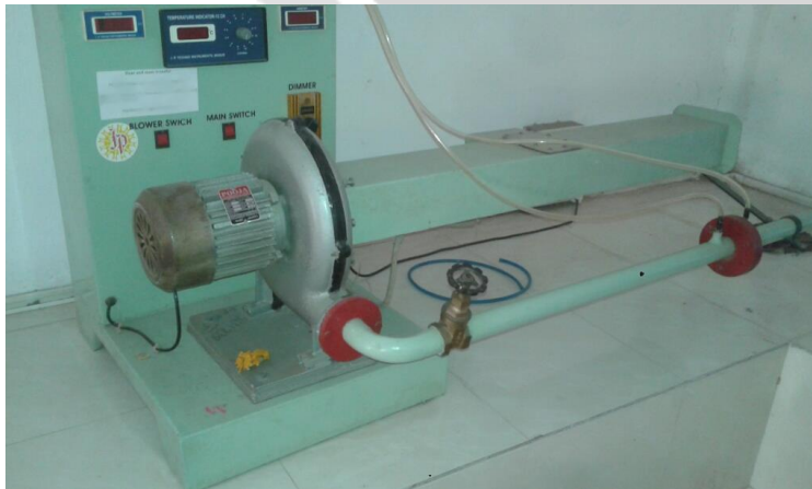
Figure 2: Experimental set-up of centrifugal blower
