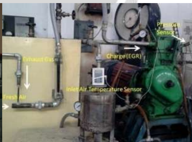
Figure 3.5: CI Engine used for Performance Analysis Figure 3.6: Photographic view of experimental setup showing EGR path
