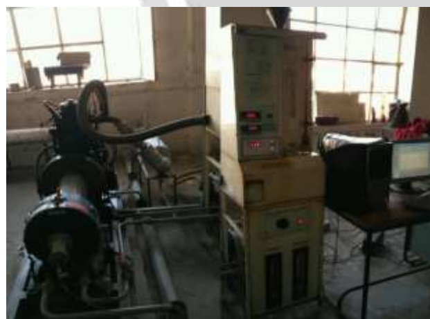
Figure 3.5: CI Engine used for Performance Analysis Figure 3.6: Photographic view of experimental setup showing EGR path
