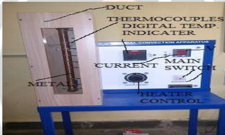
Fig. Experimental Setup Of Natural Convection
