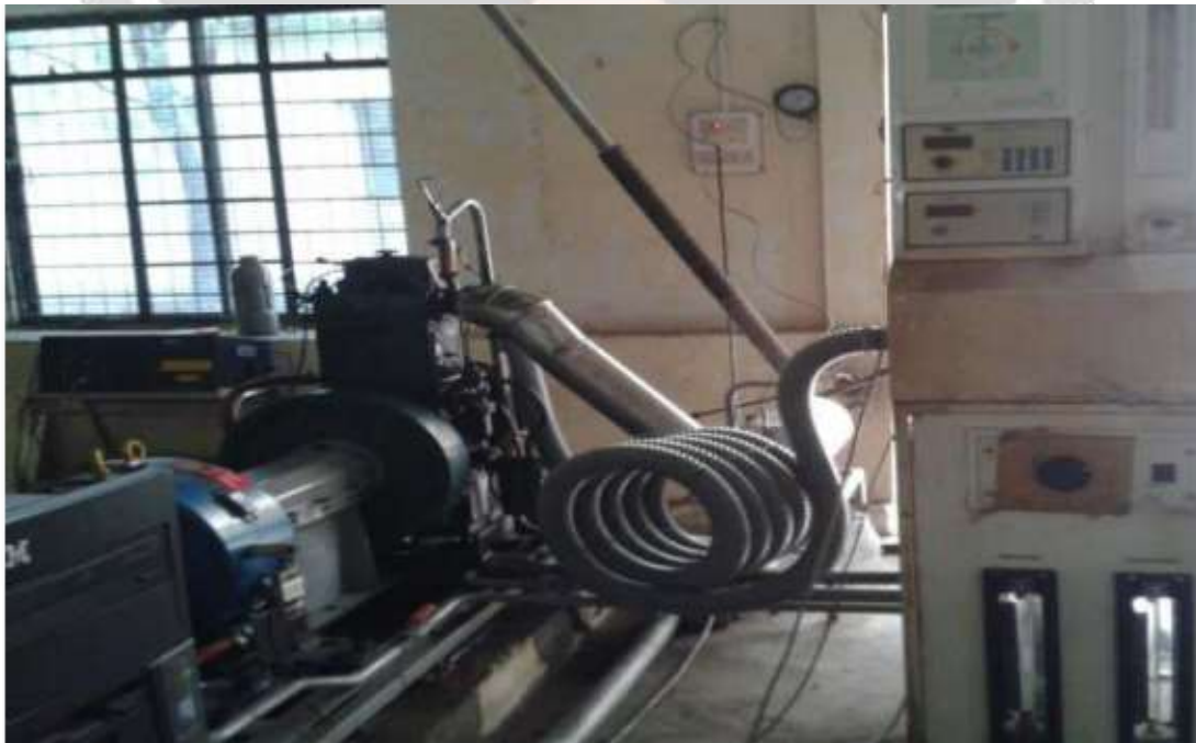
Fig: 3.2 Experimental set up with closed coil pipe connecting inlet manifold and air chamber
