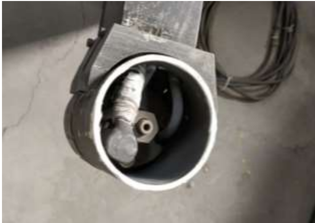
Fig.2: Welding Torch of PAW Machine (Source: Captured at Keepsake welding research & Skill development centre)
