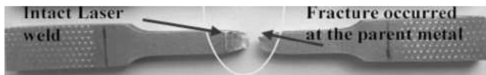
**Figure-(3)** Tensile specimen before and after conducting test
