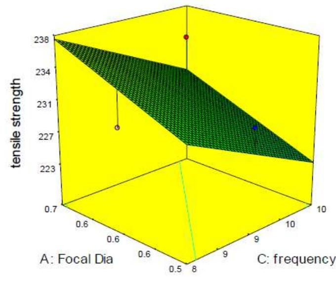
**Figure (6)** Focal Diameter Vs Frequency on tensile strength
