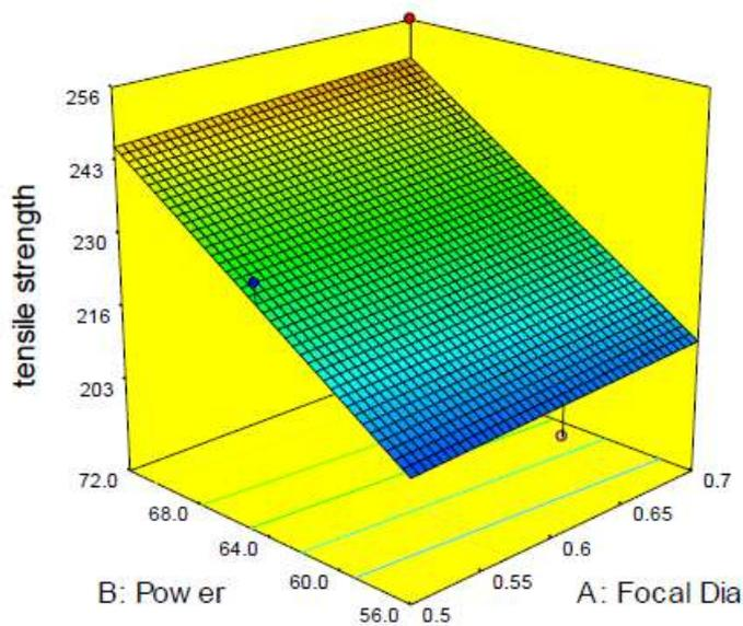
**Figure (4)** Focal diameter vs laser power on tensile strength
