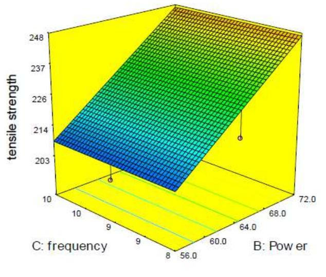
**Figure (5)** Frequency Vs Power significance on tensile strength
