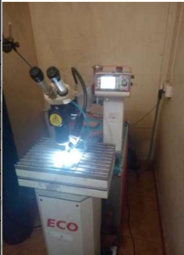
**Figure (2).** The laser beam welding machine
