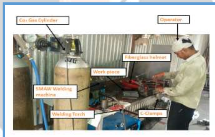
Fig. 4 Welding Machine Setup
