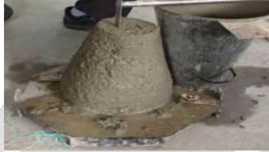
Fig -3: Slump cone test
