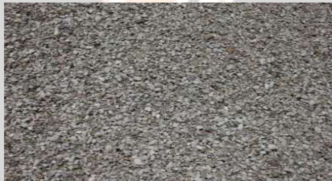
Fig- 2: Crushed Stone Sand
