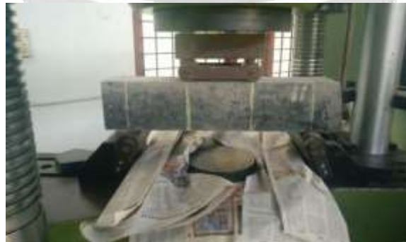
Fig -8: Flexural strength test
