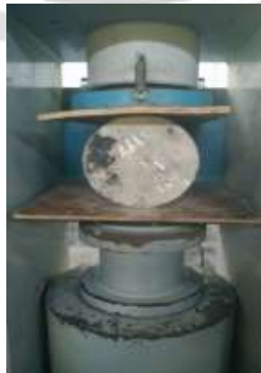
Fig -5: Split tensile strength test
