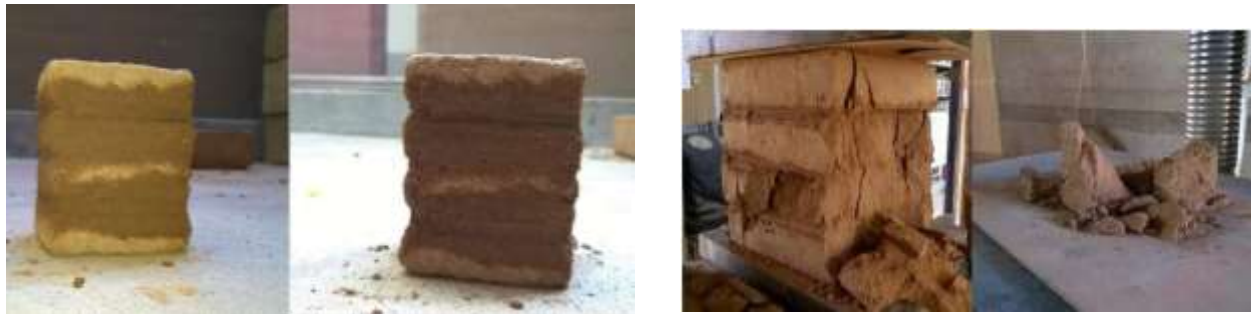
For adobe bricks, same material which was used for brick making was used as 1 cm thick mortar for prototype brick prism. While for model brick prism adobe material which was passing through 400 μm used as 2 mm thick mortar.
